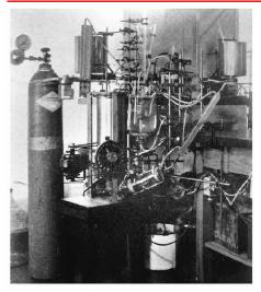
Fig 2. Photograph taken in Dr Gibbon's laboratory, showing an early version of his heart-lung machine. (Courtesy of J. H. Gibbon, Jr. Reprinted with permission from Gibbon JH et al. Arch Surg 1937; 34:1109.)
